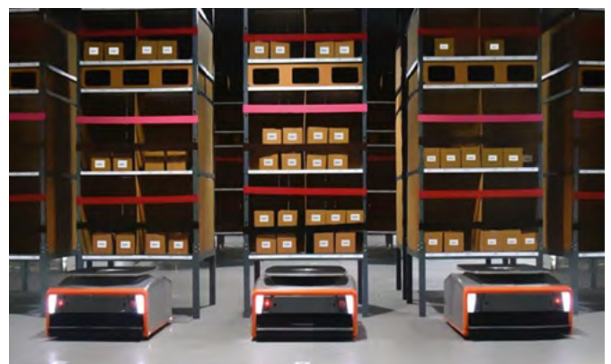
Figure 44: GreyOrange AGVs use AI-based navigation and collaboration to learn and to improve their performance over time; Source: GreyOrange
