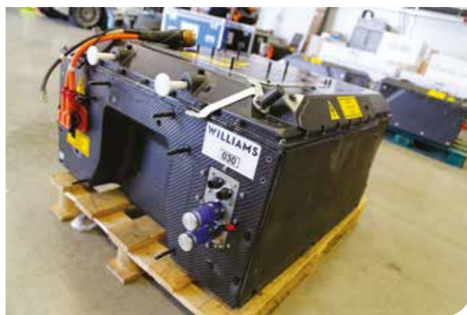
High performance Formula E racing car battery.
