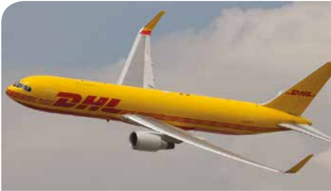
Modified Winglets of a Boeing 767.
