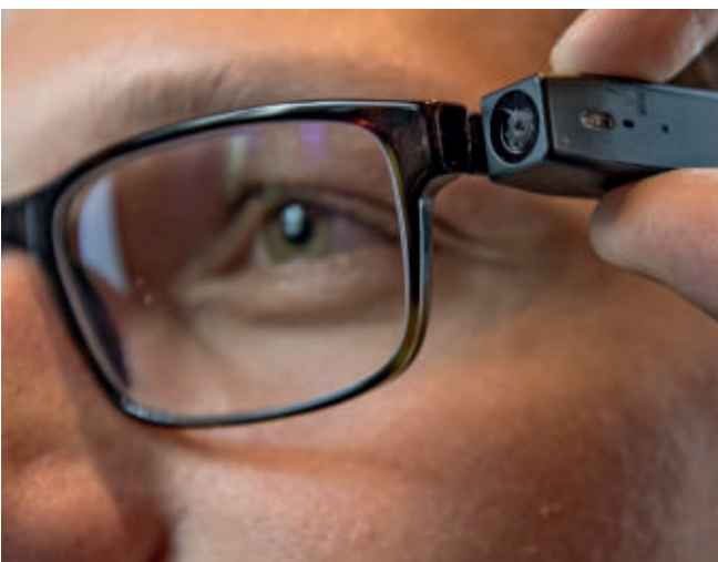
TECH SPECS: A PogoCam camera that attaches magnetically to eyewear.
