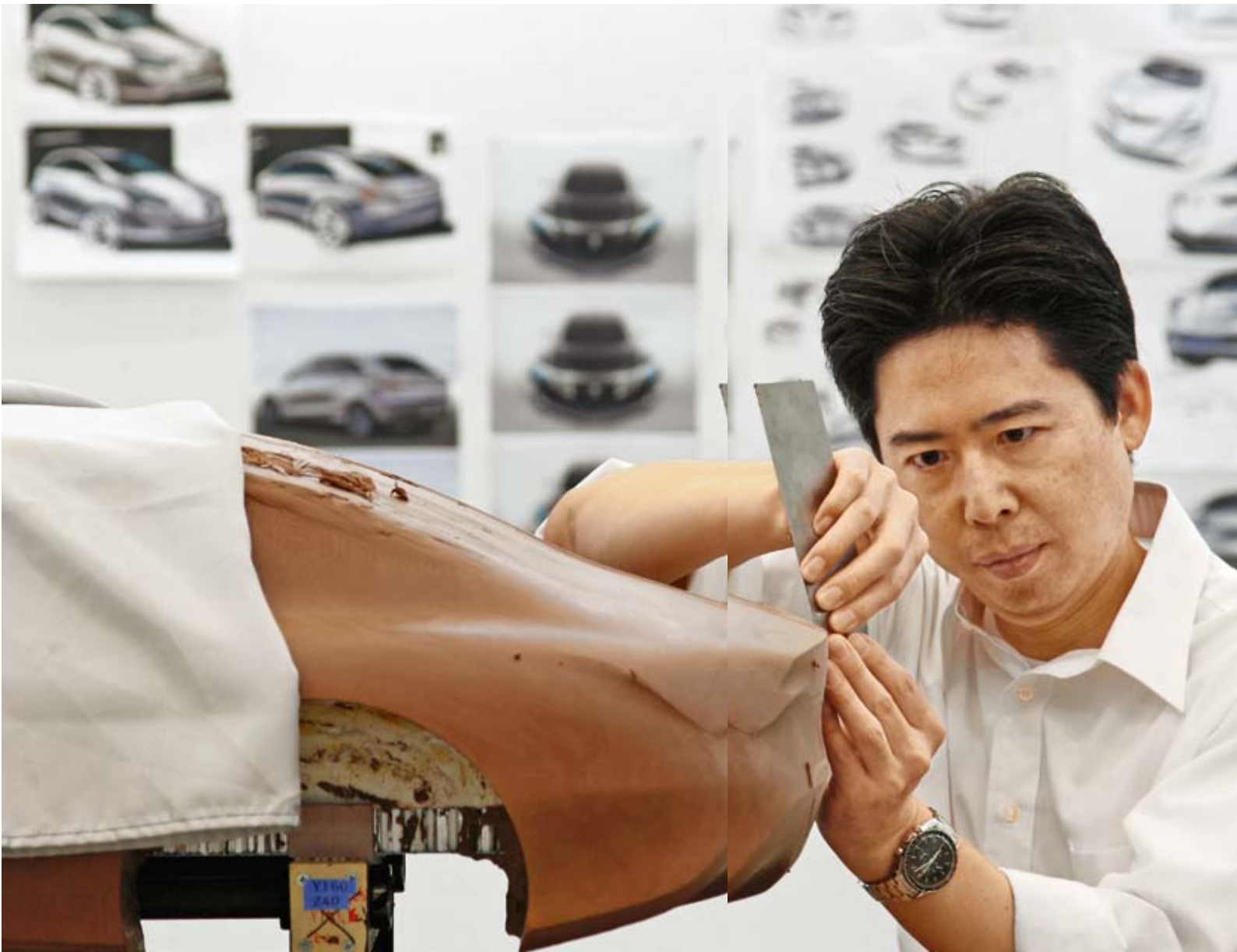
SHAPING THE FUTURE: A 1:4 clay model of a new car being formed at the Mercedes-Benz Advanced Design Studio in Tokyo, Japan.
