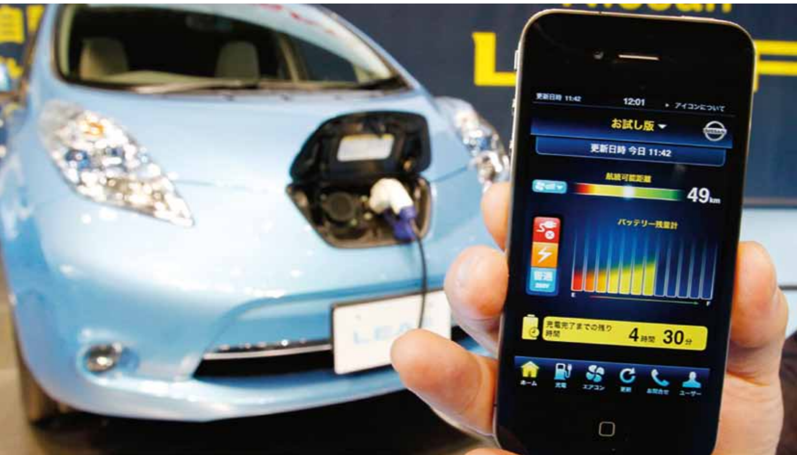
TAKING CHARGE: A smartphone app for Nissan’s LEAF allows users to start charging or check battery status remotely.
