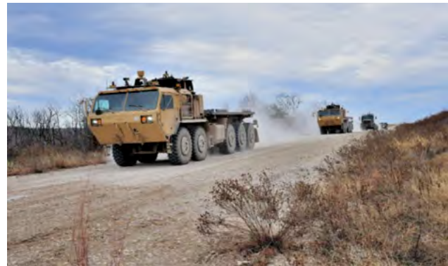
Figure 12: Driverless convoys moving through challenging terrain; Source: Foundation Media
