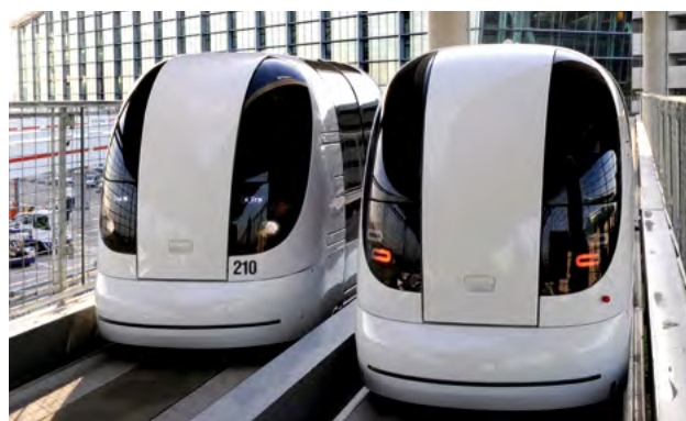
Figure 28: The Ultra Pod carrying passengers at Heathrow Airport; Source: Airspan
