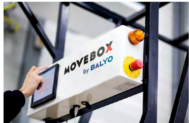
Figure 37: An ingenious way to turn a regular forklift into a self-driving vehicle; Source: BALYO
