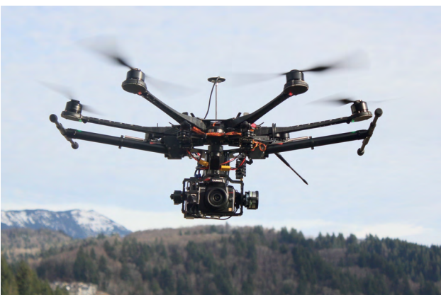
Figure 5: Multicopter used for taking low altitude aerial photos; Source: Soliforum
