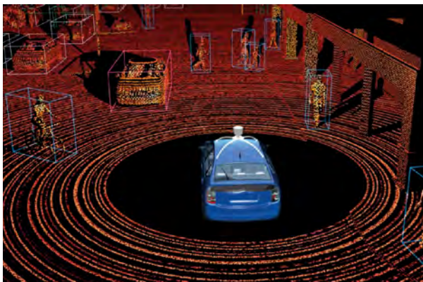
Figure 9: Using LIDAR to scan the environment; Source: DriverlessCar.com
